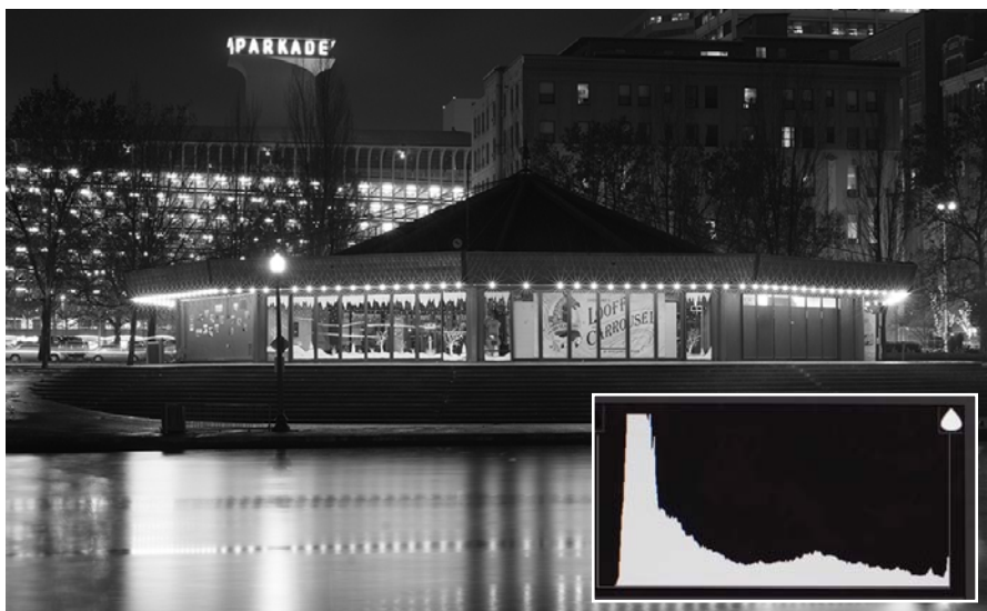
Figure 2: Original raw capture, with histogram showing brightness values.
